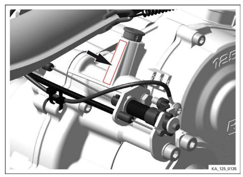
Figure 1.4: Serial number of the engine, TYPICAL
