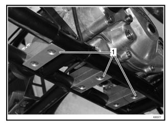
Figure 2.3: Engine brackets
