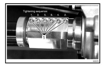
Figure 2.4: Tightening sequence
